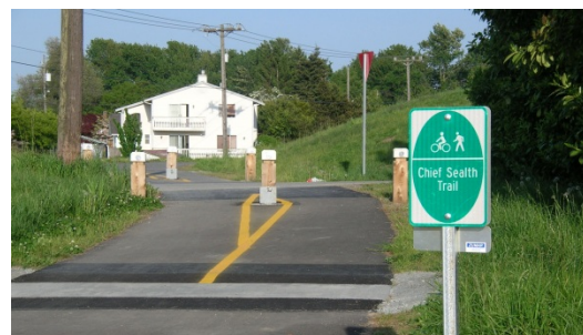
A modified M1-8a sign at the entrance to a shared use path.
