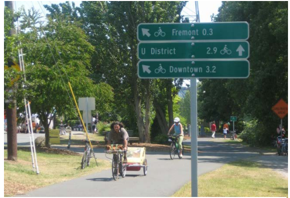
Decision and named route signs from Seattle. On paths, both sign types are used to mark the route and provide direction to destinations on and off the path.
